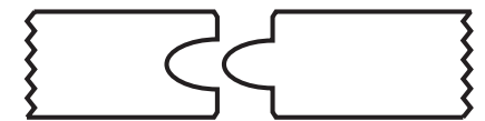
END MATCH All of our decking is end-matched for ease and improved quality of installation and to provide full coverage on or off the joist. Learn more at dassoXTR.com .
